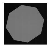
Figure 2: Representative image of the end face of an octagonal homogenizing rod showing the absence of edge defects. Image was produced using bright field illumination and 100x magnification.
