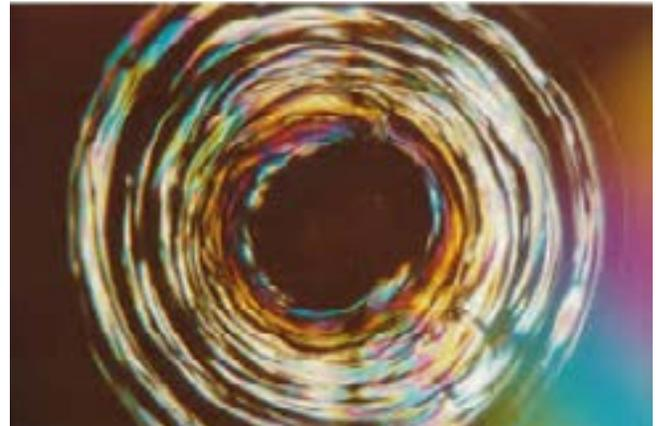
*Figure 1: Example of laser-induced damage of a high power laser optic. Source: Wikipedia.*
