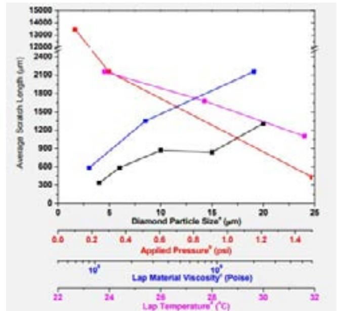
Figure 2: Relationship between average scratch length and several process parameters in polishing. Reference: Suratwala, T., 2015, "Lecture 13: Glass Finishing (Grinding & Polishing)", presentation slides, Glass Processing Course (Lehigh University; Spring 2015), International Materials Institute for New Functionality in Glass (IMI-NFG), LLNL, delivered March 5, 2015.
