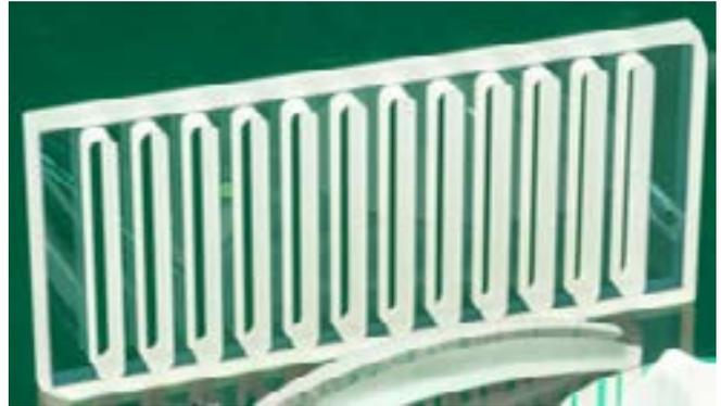
*Figure 3: Slotted high power laser mirror. Maintaining the specified clear aperture while ensuring a clean surface for coating requires close control of the bevel on the slot edges at the mirror surface.*
